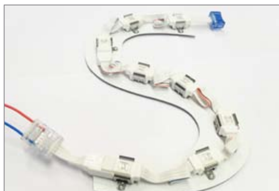
Fig. 12 LED string connected to LED Power Driver
